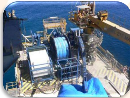
Offshore CTU installation
